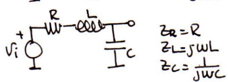
$$Z_R = R, \quad Z_L = j\omega L, \quad Z_C = \frac{1}{j\omega C}$$
