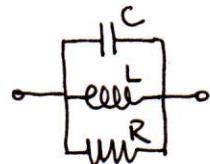
$$Y = \frac{1}{R} + j\omega C + \frac{1}{j\omega L} = \underbrace{\frac{1}{R}}_G + j \underbrace{\left(\omega C - \frac{1}{\omega L}\right)}_B$$
